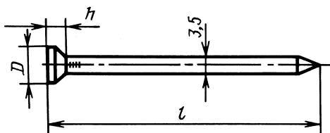
$D \text{ min} = 8 \text{ мм}; h \text{ min} = 0,6d$
